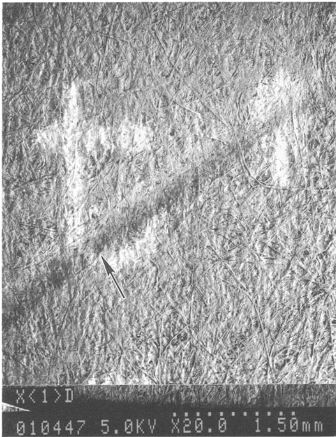
FIG. 4—@ 20X magnification. Typing first, letter “t,” then blue “BIC” ball point pen ink. Arrow indicates crossing area examined.
