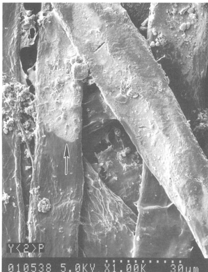
FIG. 10—@ 1000X magnification. Ball point pen “RITES” reddish/pink ink first, letter “r,” then typing. Arrow indicates crossing area examined. Note: heavy ink deposit.
