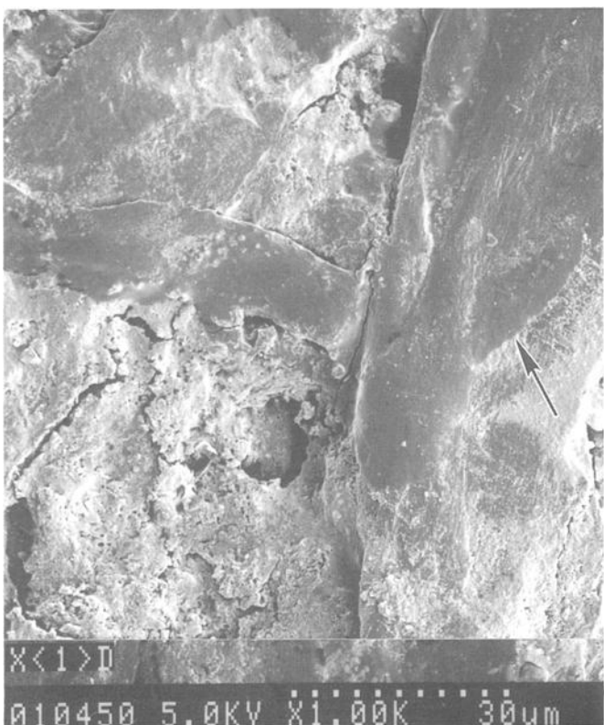
FIG. 7—@ 1000X magnification. Typing first, letter “t,” then blue “BIC” ball point pen ink. Arrow indicates crossing area examined and relates back to Fig. 6.
